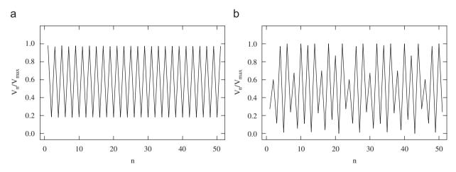
Fig. 3. The iterated map for the speed  $v_n$  at the *n*th crossing point, for: (a)  $T_{c,B}/T_{c,A} = 0.88$  and (b)  $T_{c,B}/T_{c,A} = 0.856$ , for  $x_{tol} = L_A/2$ ,  $L_A = 200 \text{ m}$ ,  $a_+ = 2 \text{ m/s}^2$ , and  $a_- = 6 \text{ m/s}^2$ . The transient has been removed.
