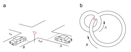
Fig. 1. (a) A sketch of the intersection to be studied: *B* is the mobile approaching the yield sign; *A* has preference to pass.  $x_d$  is the distance at which *B* must make a decision to stop or not.  $x_{tol}$  should be such that collisions are always avoided [see Eq. (1)]. (b) The roads are made to intersect at a periodic number of points.
