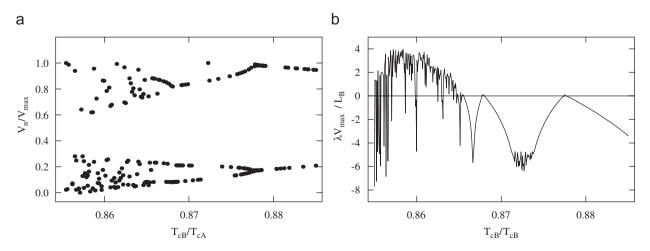
Fig. 5. The bifurcation diagram: (a) zoom of a chaotic region in Fig. 4(a), and (b) the associated Lyapunov exponent.
