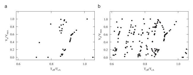
Fig. 4. The bifurcation diagram for the speed against  $T_{c,B}/T_{c,A}$  for two different values of  $x_{tol}$ , (a)  $x_{tol} = L_A/2$  (low risk of collision) and (b)  $x_{tol} = L_A/6$  (high risk). The other parameters are as in Fig. 3:  $L_A = 200 \text{ m}$ ,  $a_+ = 2 \text{ m/s}^2$ ,  $a_- = 6 \text{ m/s}^2$ . The transient has been removed.
