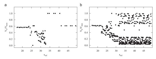
Fig. 6. The bifurcation diagram with  $x_{tol}$  for: (a)  $L_B = 152 \text{ m} (T_{c,B}/T_{c,A} = 0.760)$  and (b)  $L_B = 172 \text{ m} (T_{c,B}/T_{c,A} = 0.862)$ .
