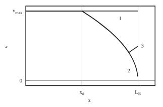
Fig. 2. Possible situations for *B* at the decision point  $x_d$ , namely: (1) continuing, (2) braking to stop at  $x = L_B$  before *A* leaves the crossroad, and (3) braking and accelerating again as *A* leaves the crossroad before *B* stops completely.
